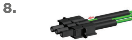
Slide shrinking tube (1) on connector shell (3)
