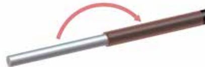
Fold back shield braid over jacket
