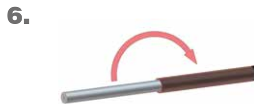
Fold back shield braid over jacket
