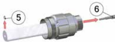
Remove snap ring (5), take out male contact (6) from insulation part (4)
