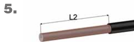
⚠ ONLY when using shielded cable: Remove cable jacket
